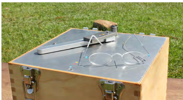
The bending unit – this wooden box contains a complete opticians’ workshop. | © Martin Aufmuth
